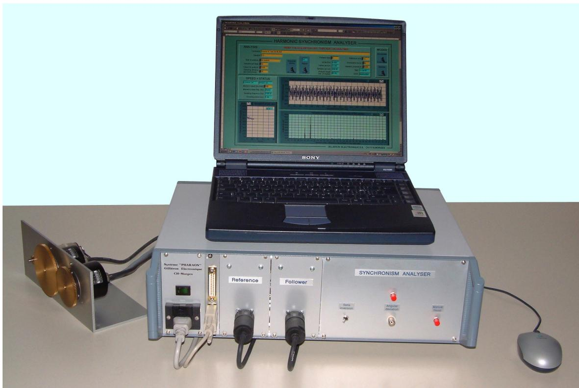
***The synchronism analyser with the test and demonstration equipment***
